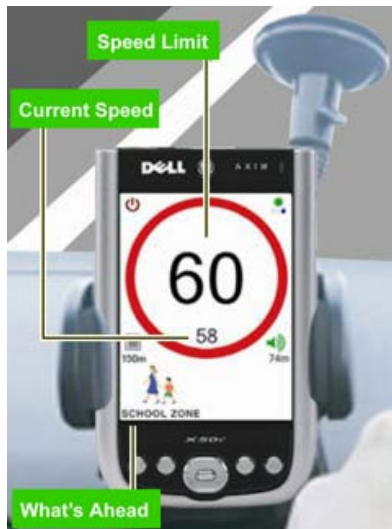
Figure 2.7: SpeedAlert working on a PDA or mobile phone (source: Smart Car Technologies)
