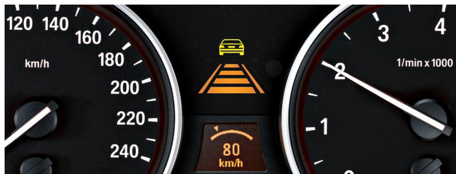
Figure 2.5: Dashboard indicator showing Stop & Go enabled and tracking a vehicle ahead (source: BMW)
