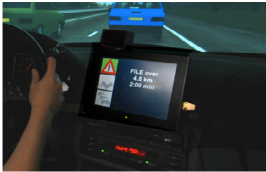
Figure 6.1: Display of the Congestion Assistant on the centre console
